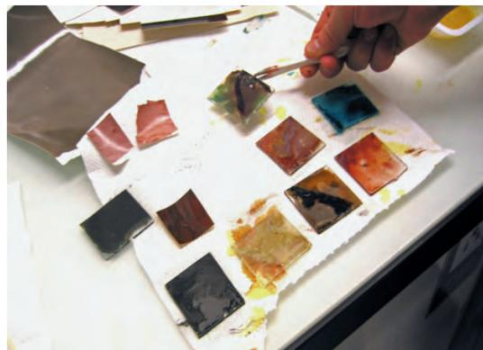
Samples of paint on glass supports in the Laboratory of Inorganic Chemistry at ETH Zurich
